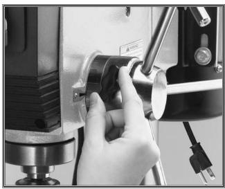
Figure 26. Loosening collar lock knob.
